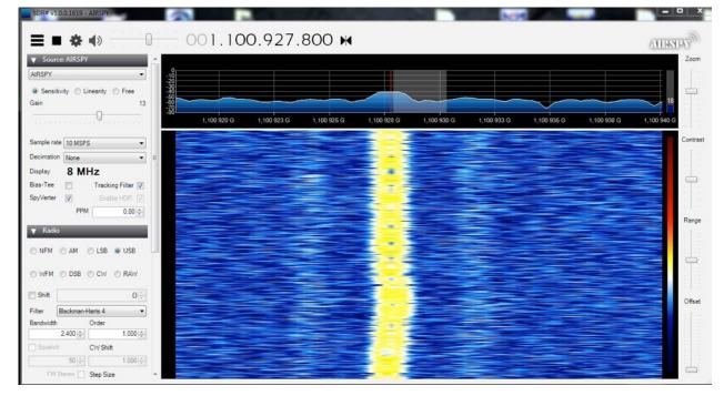
Its a good Practice that you have your RX and TX Frequency adjusted so it DISPALY the same Frequency in your SDR Software. In reality the upper Beacon would be at 10.489800 GHZ. When we would THEORETICALLY want to send on the Beacons Frequency we would have to set our TX Frequency at 2.400300GHZ. I'd suggest you send your RX Frequency in your SDR Software so it matches the actual TX Frequency. It makes Things much easier...
