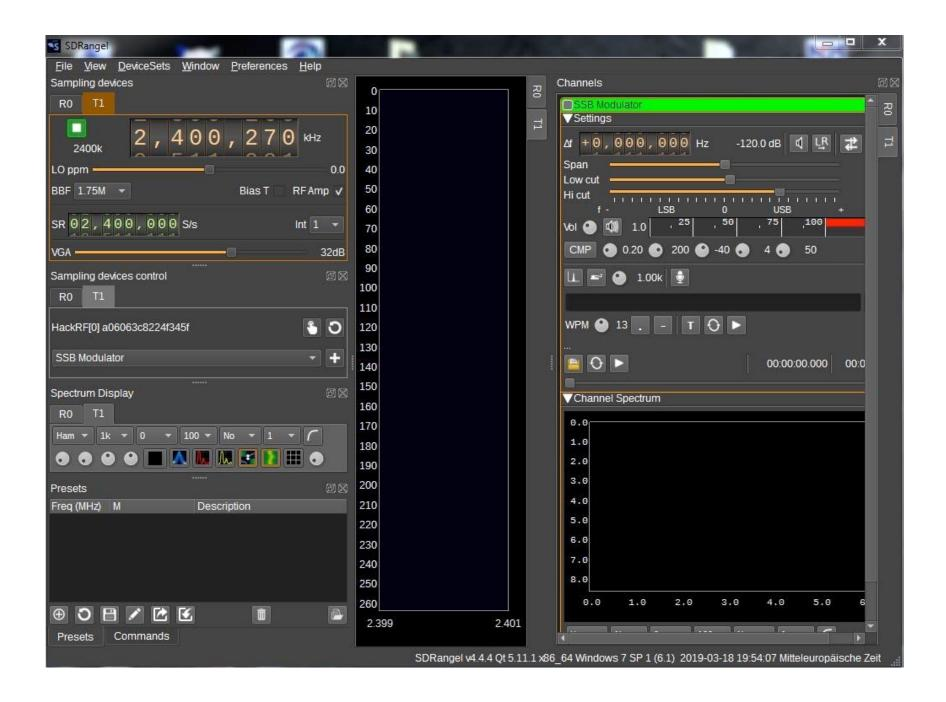
On the Right side of the Window there is in the a Button showing a "Amplitude" on a Graph. If you press this Button the SDR will send a Carrier Signal.
