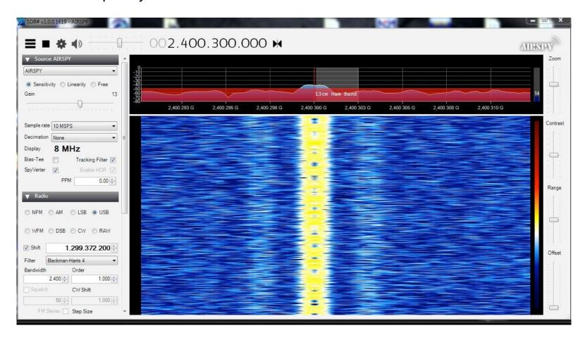
You can doublecheck your Offset by centering your RX Frequency at the lower CW Beacon. The Readout should be 2.400050GHZ
